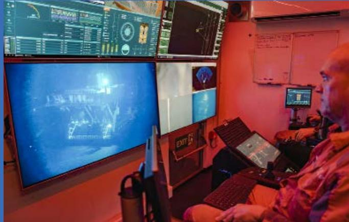
The nodule-collecting machine gets lowered to the ocean floor on a cable that's nearly 3 miles long. Onboard the ship, engineers in a control room monitor its progress.
