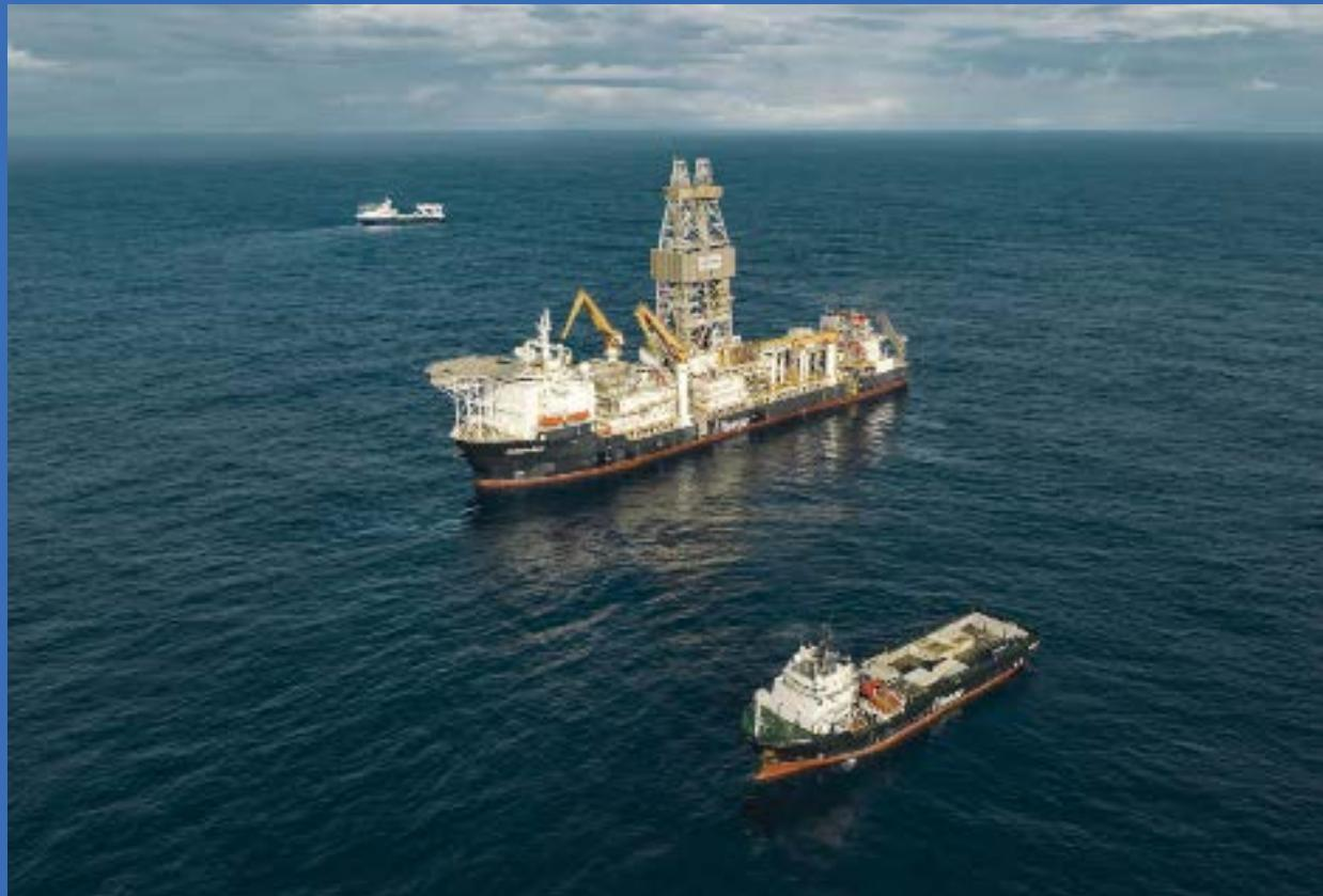
The Metals Company uses a former oil-drilling vessel, the *Hidden Gem*, to collect polymetallic nodules from the seafloor.
