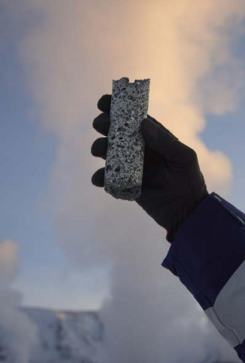
IN ICELAND AND ELSEWHERE, CAPTURED CARBON CAN BE INJECTED UNDERGROUND, TURNED INTO ROCK, AND STORED LONG-TERM.
